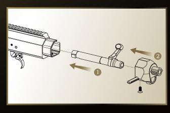
1.Insert the bolt into the upper receiver. 2.Install the stock adapter.
