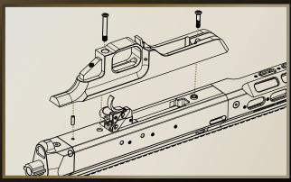
Assemble the upper receiver with the lower receiver.
