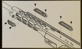
Set the side rail on the receiver and the handguard.
