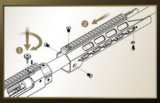
1.Fasten the knob. 2.Assemble the handguard with the upper receiver.
